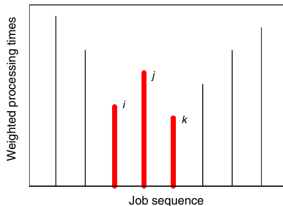
Fig. 1. An illustration of V-shape violation.
