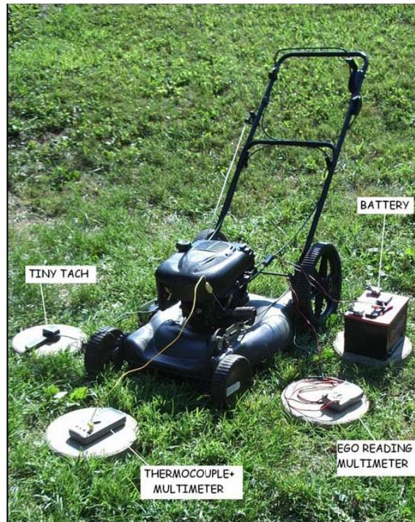
Figure 1) Test Setup of Lawn Mower.
