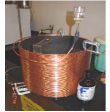
Copper Tube wound on a drum prior to filling with LMA
