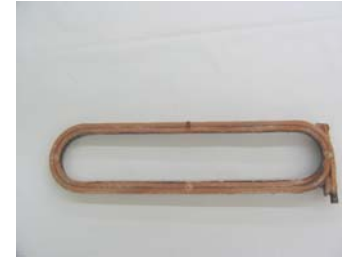
Epoxy impregnated coil removed from the winding form
