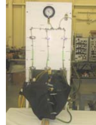
R&D coil in thermal blanket during epoxy impregnation
