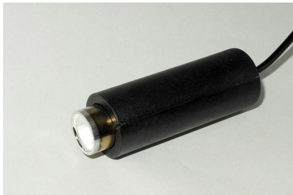
Figure 13. End-window Geiger-Mueller tube for detecting and counting diffracted x-rays.
