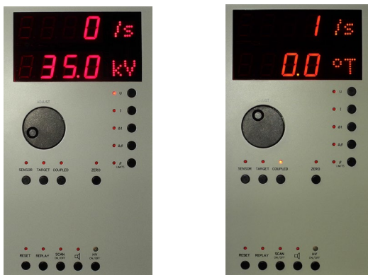
Figure 7. Leybold Didactic (LD) x-ray diffraction system control panel.
