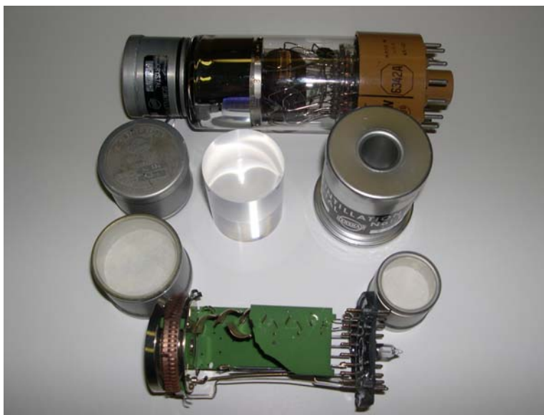
Figure 4. A picture of a photomultiplier tube, several examples of NaI and plastic scintillators and, the insides of a photomultiplier tube showing the curved dynodes.
