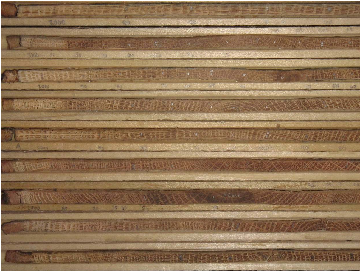
Figure 4.2 Oak increment cores were mounted, sanded, and dotted before measurement.
