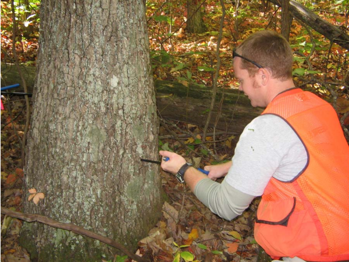
Figure 4.1 An increment borer is used to extract a core sample from a black oak.
