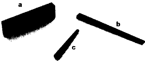
Figure 3. The three types of stones used to sharpen increment borers: (a) the larger flat stone, (b) the tapered sharpening stone, and (c) the conical stone.
