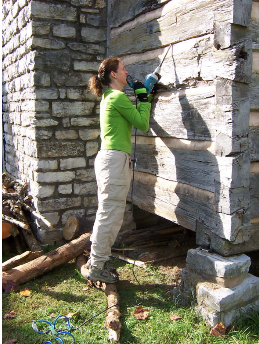
Figure 3. Extracting a core from the Walker Springs cabin (east side, log WSE04, basal end) using an electric drill and the specially-designed hollow corer.
