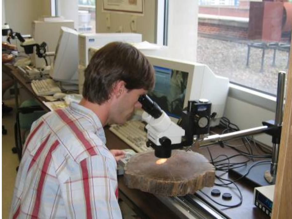
FIGURE 4. J.L. Hart measuring the widths of tree rings on a cross section from the Hope Mills crib dam. This process took several months due to the lengths (i.e. extensive ages) of the tree-ring series on these longleaf pine sections.
