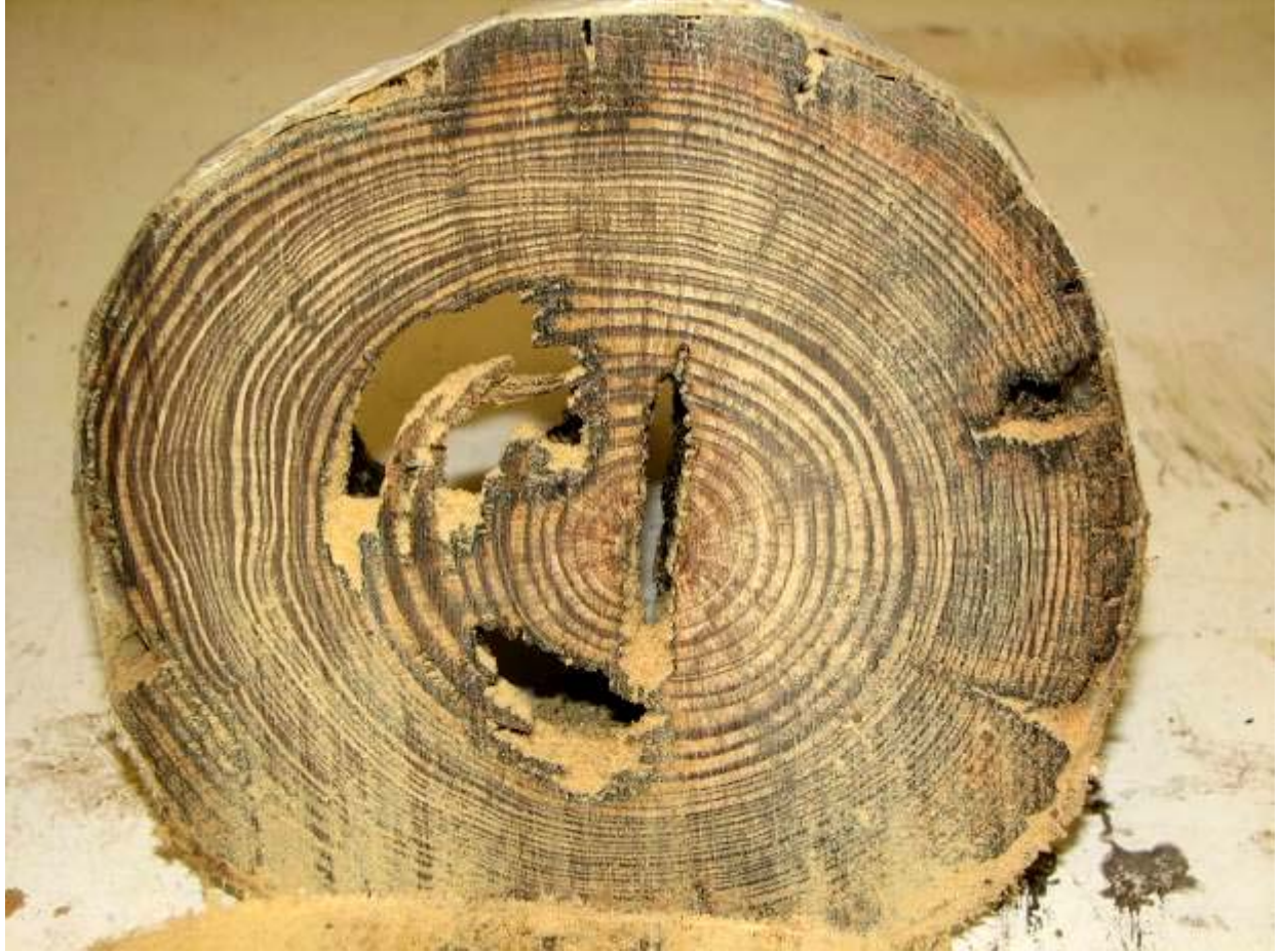
Figure 2. Pine sample 8SJ31-2741 after being sawn to reveal the interior ring structure.
