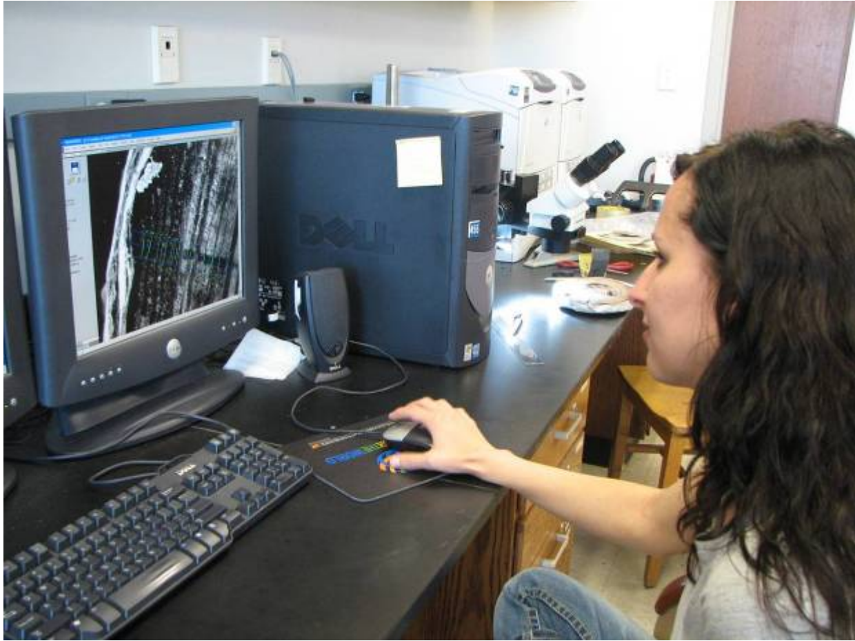
Figure 3. Operating WinDendro to measure the ring widths of pine sample 8SJ31-2741 in the Laboratory of Tree-Ring Science.
