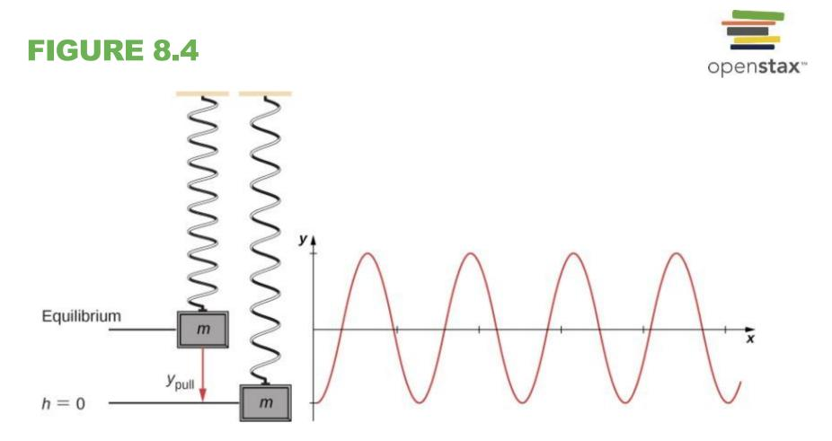
A vertical mass-spring system, with the *y*-axis pointing upward. The mass is initially at an equilibrium position and pulled downward to  $y_{pull}$ . An oscillation begins, centered at the equilibrium position.
