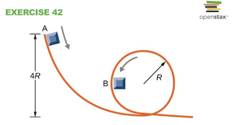
A small block of mass m slides without friction around the loop-the-loop apparatus shown below. (a) If the block starts from rest at A, what is its speed at B? (b) What is the force of the track on the block at B?
