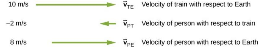
Velocity vectors of the train with respect to Earth, person with respect to the train, and person with respect to Earth.
