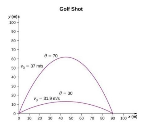
Two trajectories of a golf ball with a range of 90 m. The impact points of both are at the same level as the launch point.
