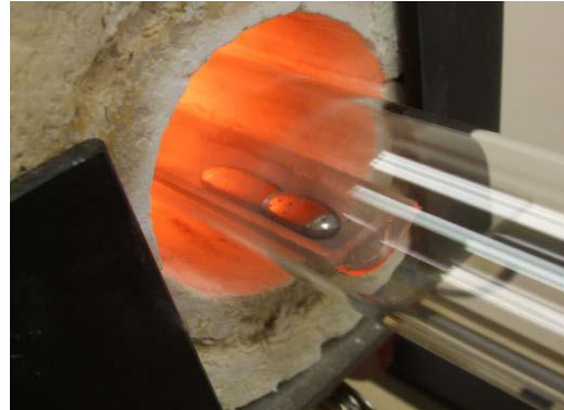
Reduction to Ge metal at Electrochemical Systems Inc. (ESI)
