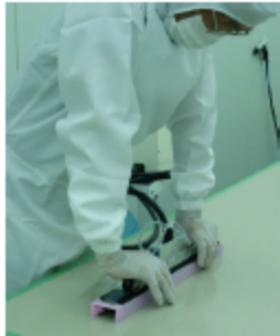
Welding gores by an impulse welding machine
