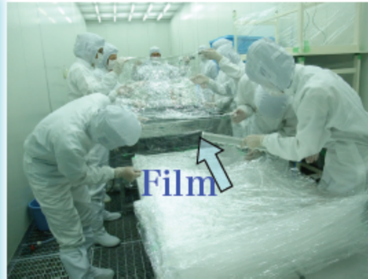
Film rinsing with ultra-pure water using an ultrasonic machine
